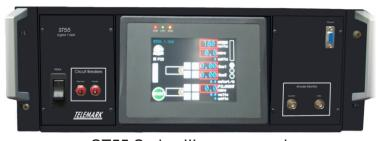
ST55 Series III power supply with tilting Touch Screen interface
